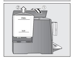
Open the lid on the left hand side of the coffee system ①. Pull the water tank up and out using the handle ②. ■ Fill the water tank with fresh, cold tap water to the "Max." mark.
